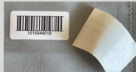
Place Label with barcode facing fabric with arrows up before Heat Seal Application of Label.
