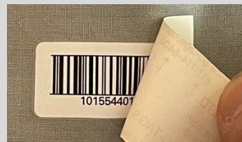
After heat seal application, remove paper backing.
